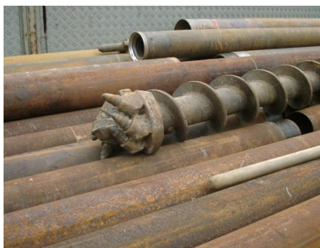
Figure III-2.2-ii.13d-h: Examples of cased auger/pulse drill required for Hard ground and rock drilling
