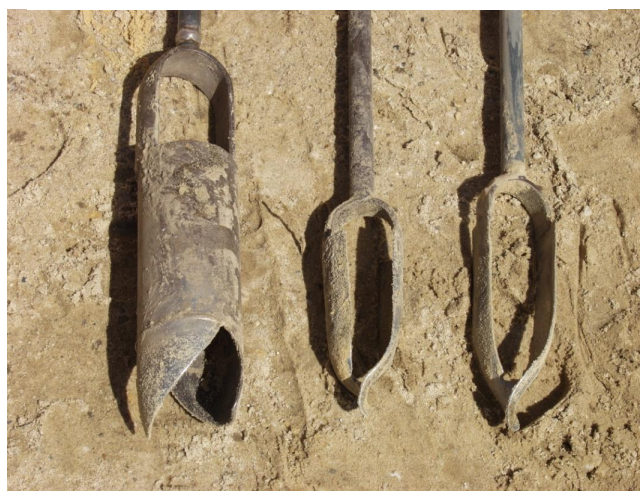
Figure III-2.2-ii.5b Example of augers. From left to right: Riverside (gravel, debris), auger (sand), Edelman auger
