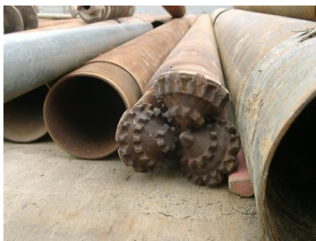
Figure III-2.2-ii.13d-h: Examples of cased auger/pulse drill required for Hard ground and rock drilling
