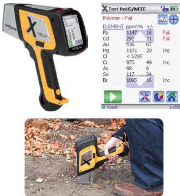
Picture 2. The Olympus Delta portable X-Ray Fluorescence Analyser with screen shot example of digital screen readout for metals in polymer. Source: www.innovx.com
