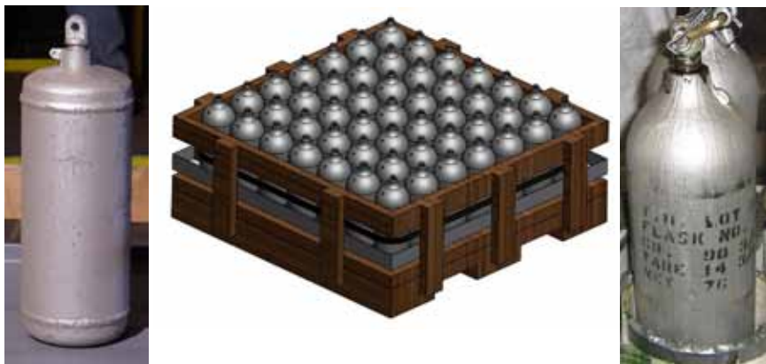
Picture 16. Examples of mercury packaging - standard 3 litre elemental mercury flasks individually and packed in a 49 x 3 litre crate with built-in spill tray. Source: US DoE 2009
